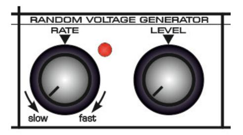
This circuit produces a stepped random voltage. The same as when you clock and feed noise through a sample and hold.
