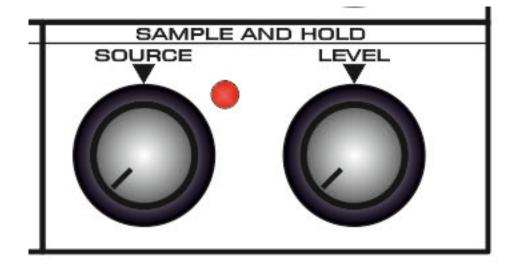
A sample and hold will 'sample' the input voltage, and hold it a static level. The sample takes place each time a clock signal is received.
