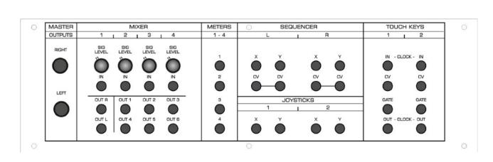
The jack panels require mono 3.5mm jack plugs. It's not possible to fit all the signals on the matrix panels, there are simply too many. So nearly every signal is also available on the jack panels.
